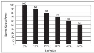
That is, if you select a value of 10% by adjusting the knob, the servo amp. will reduce the power by 10% and output only 90% of the maximum torque in overloaded situation. You can set the value between 10% and 50%. If you select "Off" in this mode, overload protection will not be activated, and the servo will always produce maximum torque. When the overload is released, the protection mode is terminated and the servo will work normally
